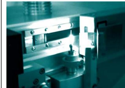
MiniVID as a stand-alone camera. Capillaries at 1500 K, heated by a diode laser.
